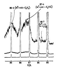
Figure 2. Metastable peaks for the transitions  $M^+ \rightarrow M - C_2H_2$ (*m/e* 89.0),  $M^+ \rightarrow M - C_2HD$  (*m/e* 87.4) and  $M^+ \rightarrow M - C_2D_2$ (*m/e* 85.7) in the 70-eV spectrum of benzothiophene-2,3-d<sub>2</sub> (11).
