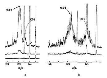
Figure 1. (a) Metastable peaks for the transitions  $M^+ \rightarrow M - HCN$ (*m/e* 103.8) and  $M - H \rightarrow M - H_2CN$  (*m/e* 102.9) in the 70-eV spectrum of  $\alpha$ -cyanonaphthalene. (b) Metastable peaks for the transitions  $M^+ \rightarrow M - HCN$  (*m/e* 105.8) and  $M^+ \rightarrow M - DCN$ (*m/e* 104.0) in the 15-eV spectrum of 1-cyanonaphthalene-2,4-d<sub>2</sub> (9).
